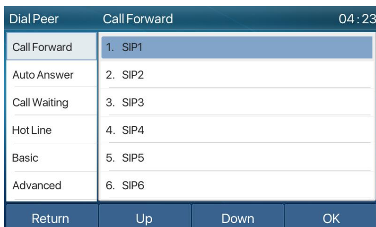
Picture 40 - Select the line to set up call forwarding
